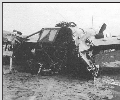
This B-26 crashed on takeoff and broke in half at the gunner's compartment.
