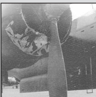
This B-26 hit a cable stretched across a valley by the North Koreans to bring down our low flying planes, but he made it back to K-8.
